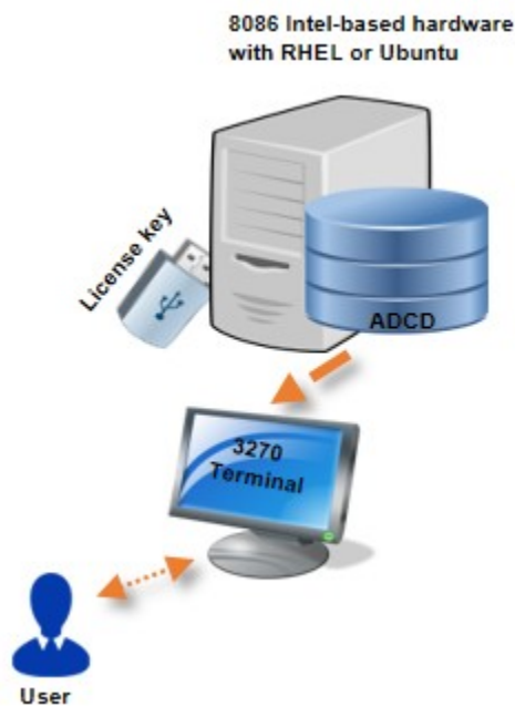
Figure 1. The topology and various components of Learners Edition
