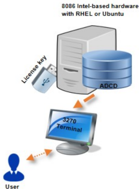
Figure 3. The topology and various components of Personal Edition
